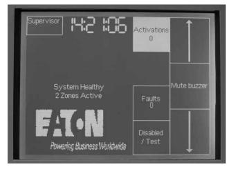
At the end of this boot sequence, all LEDs are tested, and the display shows the first entry screen.
