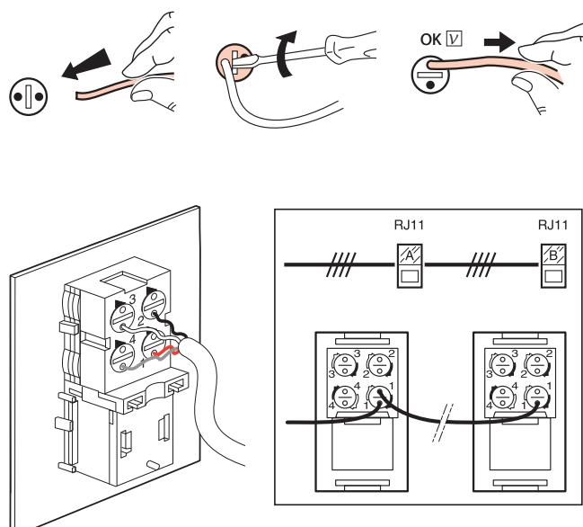
**RJ11 socket****Technical characteristics****- Protection index:**
