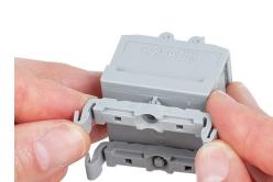
Snapping a mounting foot (209-120) to a terminal strip with snap-in mounting feet. (Distance between mounting feet: approx. 20 ... 25 mm)
