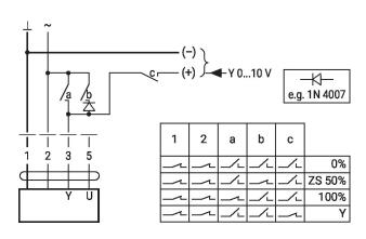
Override control with AC 24 V with Control remotely 0...100% with rotary switch
