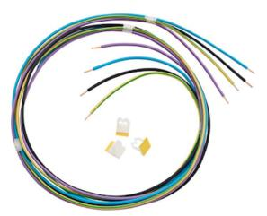
Through wiring kit for Optix Linear luminaires. Contains 4x1.5mm2 wires and self adhesive mounting clips to power constant current and emergency luminaires. Use this kit with standard luminaires as well if mounted in line with emergency versions. Length 1500mm.
