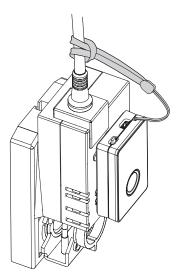
**Note** The ZIP-BT-NFC should be secured to the device with the retaining strap to avoid injury and damage to personnel and property.
