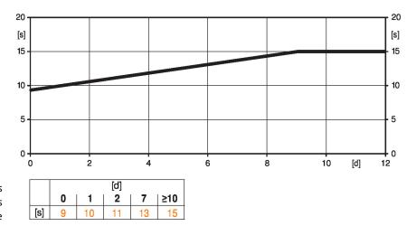
[d] = Power failure in days [s] = Pre-charging time in seconds PF[s] = Bridging time
