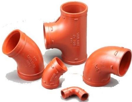
Shurjoint ductile iron grooved-end fittings are made of ductile iron per ASTM A536 Gr. 65-45-12. C-E dimensions are manufacturer's standard.
