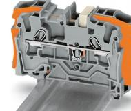
**Step-down jumper (Item No. 2006-499)** commons 6/4 mm<sup>2</sup> (10/12 AWG) terminal blocks (2006/2004 Series) with 4/2.5/1.5 mm<sup>2</sup> (AWG 12/14/16) terminal blocks (2004/2002/2001 Series).
