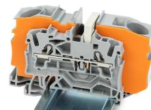
**Step-down jumper (Item No. 2016-499)** commons 16/10 mm<sup>2</sup> (16/8 AWG) terminal blocks (2016/2010 Series) with 10/6/4/2.5 mm<sup>2</sup> (8/10/12/14 AWG) terminal blocks (2010/2006/2004/2002 Series).
