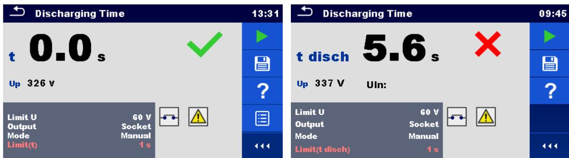
Figure 4.48: Examples of Discharging Time measurement results (Output = Socket)
