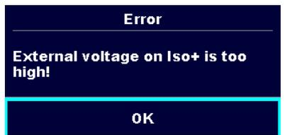
In pre-test a too high external voltage was detected between ISO/SUB and PE terminals. The measurement was cancelled. Press OK to continue.
