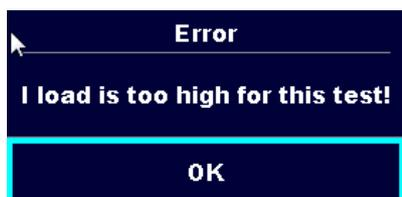
The load current exceeded the highest upper limit of 10 A for the Discharging time test. Press OK to continue.
