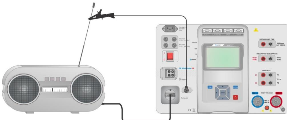
Figure 4.26: Measurement of Sub-leakage, Sub-leakage-S (socket)
