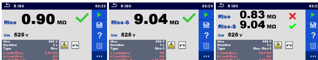
Figure 4.22: Examples of Insulation resistance measurement results
