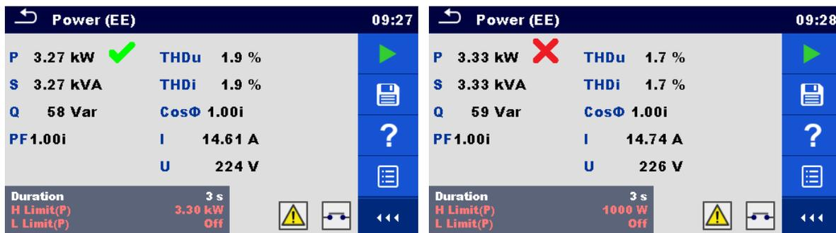
Figure 4.39: Examples of Power measurement results
