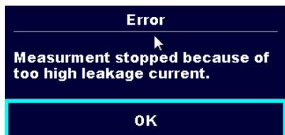
The measured leakage (I<sub>diff</sub>, I<sub>pe</sub>, I<sub>touch</sub>) current was higher than 20 mA. Measurement was aborted. Press OK to continue.
