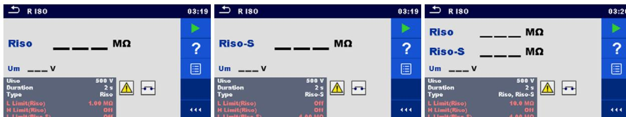
Figure 4.18: Insulation resistance test menus
