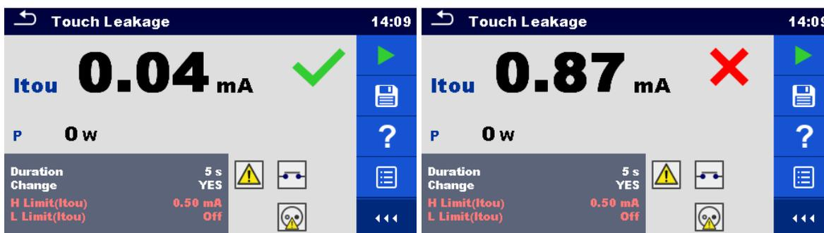
Figure 4.36: Examples of Touch Leakage measurement results
