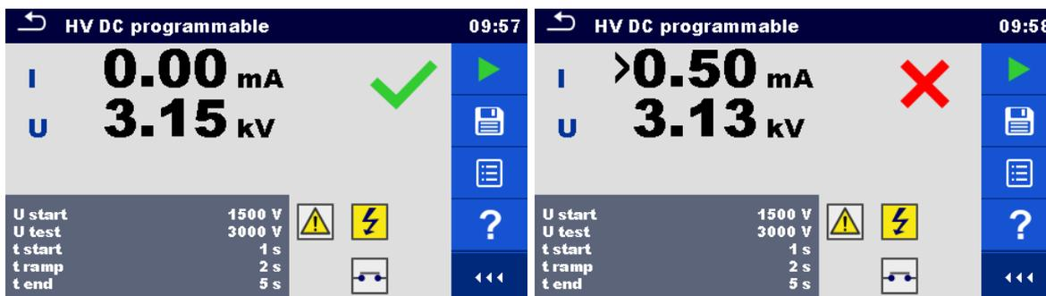
Figure 4.17: Examples of HV DC programmable test results
