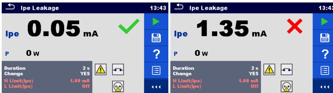
Figure 4.33: Examples of Ipe Leakage measurement results
