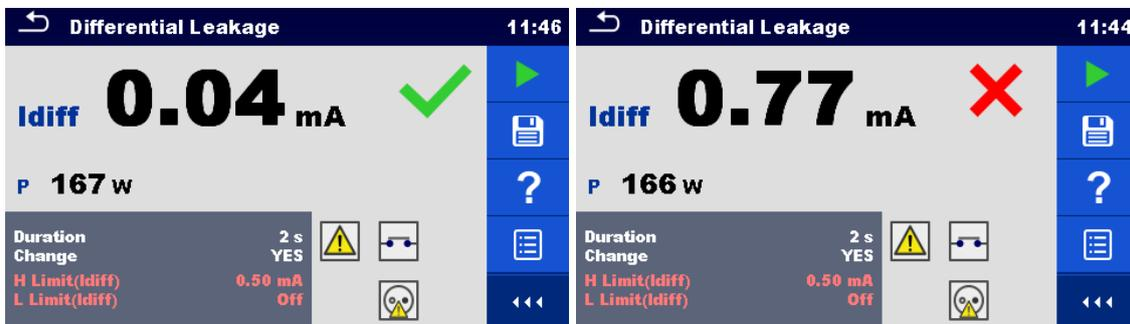
Figure 4.30: Examples of Differential Leakage measurement results
