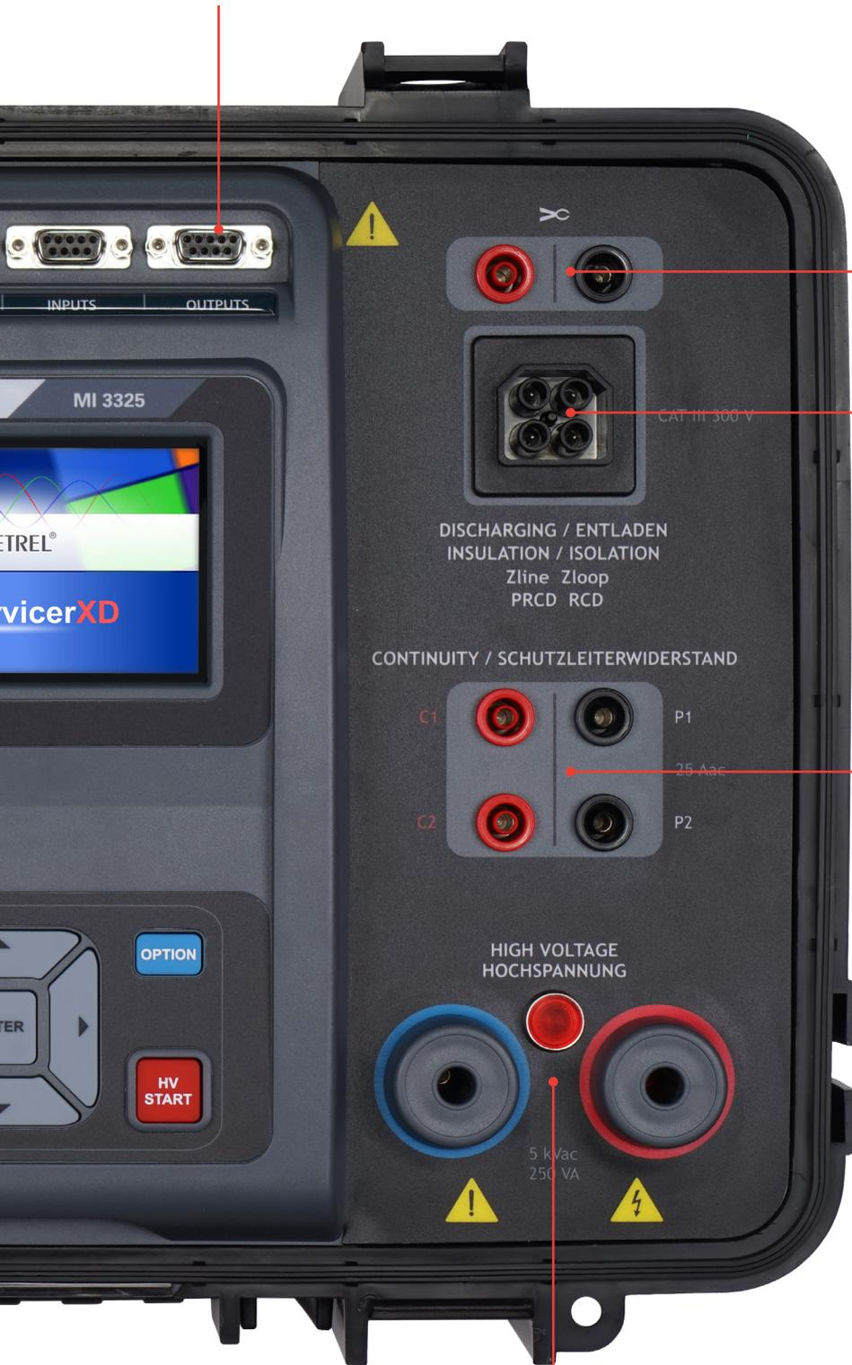
Connection ports for A 1579 Leakage current clamp
