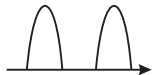
Pulsating current with DC components can be detected by type A and F RCDs
