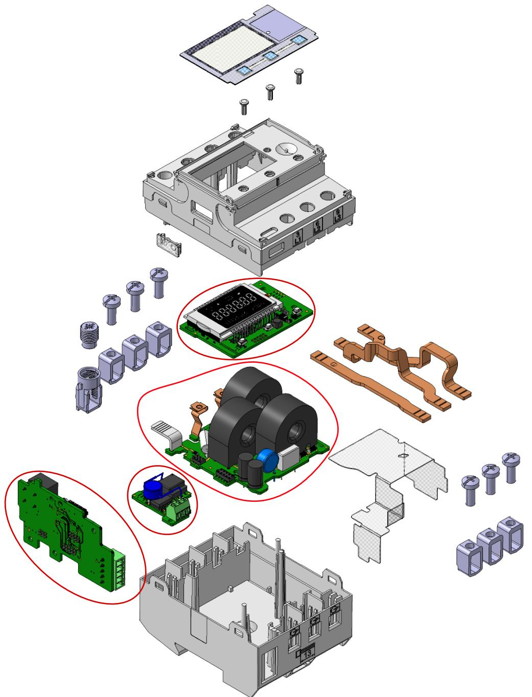
\*Rounded parts have soldered or riveted pieces that cannot be manually disassembled.
