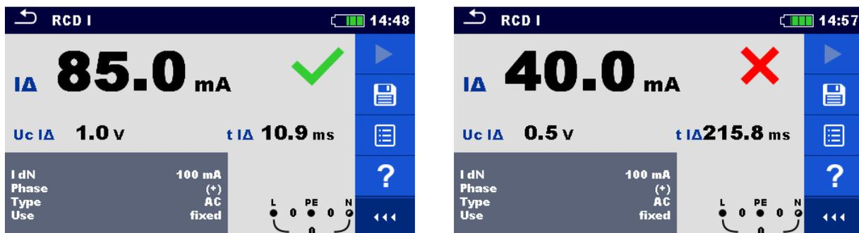
Figure 7.26: Examples of Trip-out current measurement result
