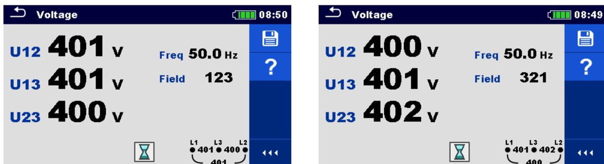
Figure 7.5: Examples of Voltage measurement in three-phase system
