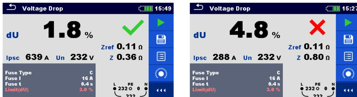
Figure 7.47: Examples of Voltage drop measurement result (STEP 2)
