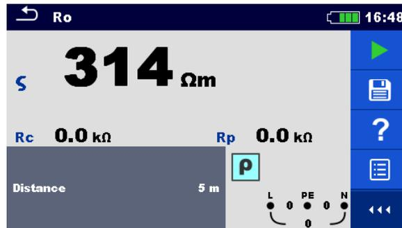
Figure 7.57: Example of Specific earth resistance measurement result
