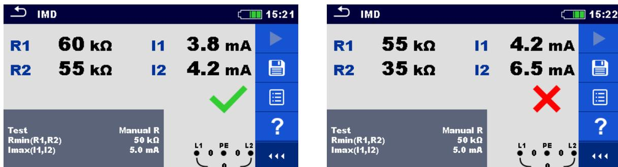
Figure 7.73: Examples of IMD test result
