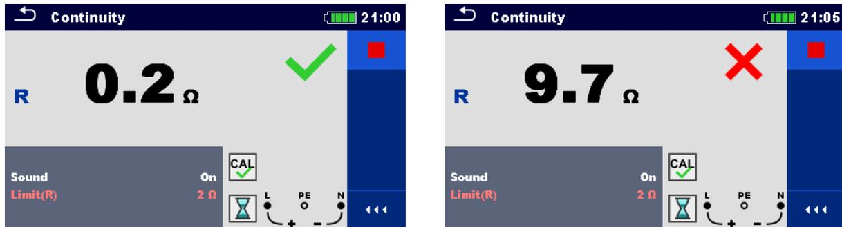
Figure 7.19: Examples of Continuity resistance measurement result
