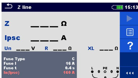
Figure 7.38: Z line measurement menu
