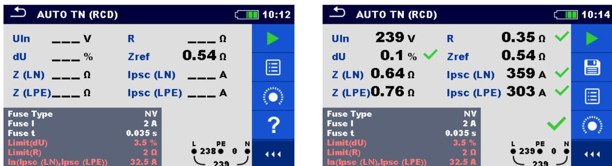
Figure 8.8: Examples of AUTO TN (RCD) measurement results
