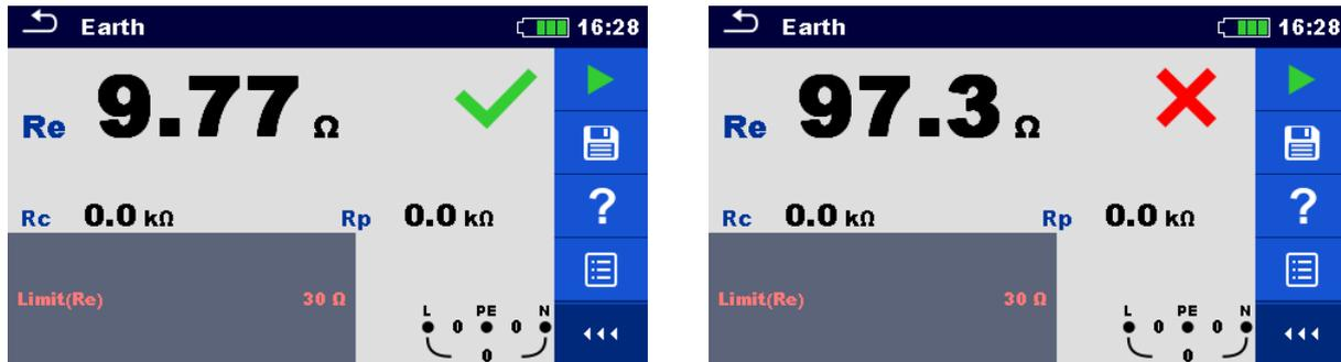
Figure 7.51: Examples of Earth resistance measurement result
