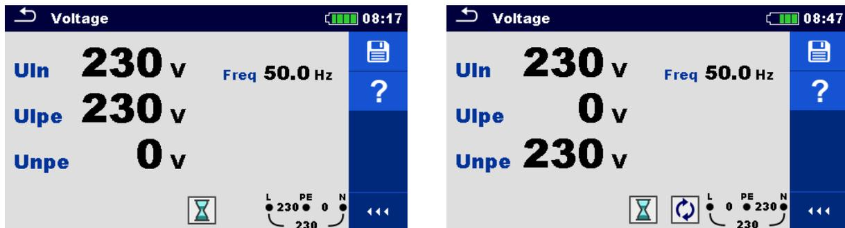
Figure 7.4: Examples of Voltage measurement in single-phase system
