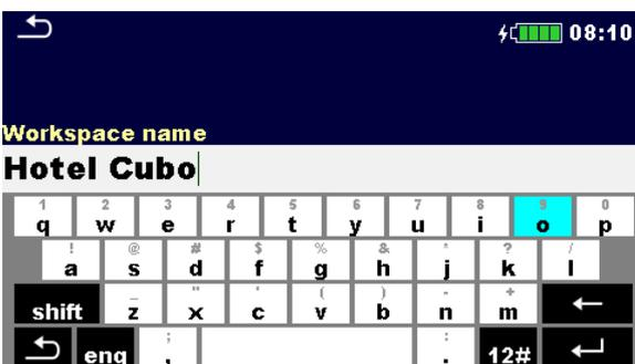
Keypad for entering name of a new Workspace is displayed after selecting New.
