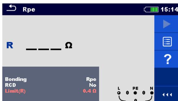
Figure 7.74: PE conductor resistance measurement menu
