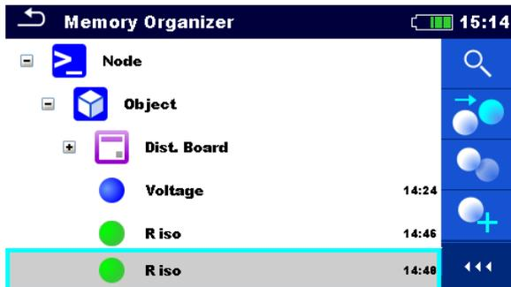
Retested measurement is saved under same structure object as original one.
