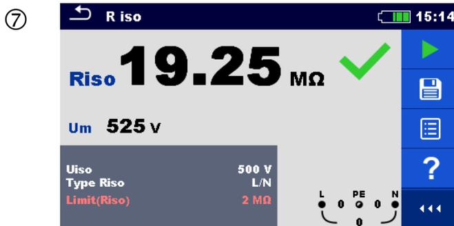
Results / sub-results after re-run of recalled measurement.
