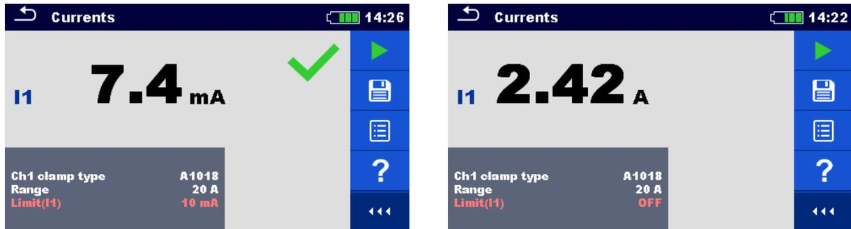
Figure 7.66: Examples of Current measurement result
