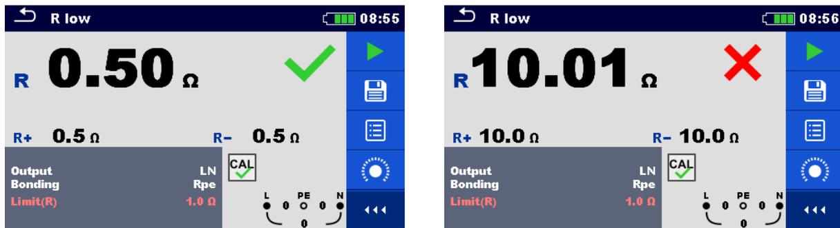
Figure 7.16: Examples of R low measurement result
