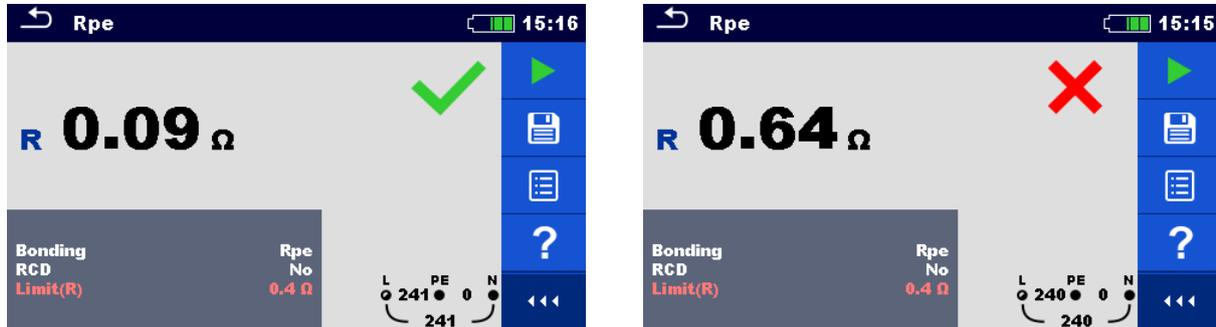
Figure 7.76: Examples of PE conductor resistance measurement result
