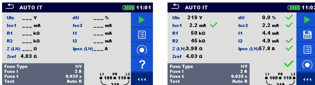
Figure 8.14: Examples of AUTO IT measurement results
