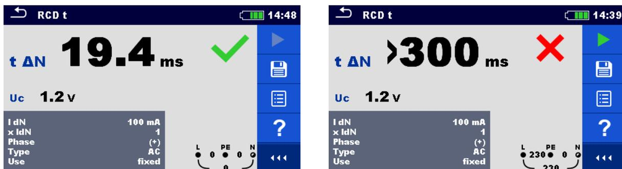
Figure 7.25: Examples of Trip-out time measurement result
