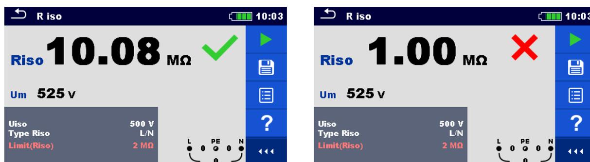
Figure 7.9: Examples of Insulation resistance measurement result
