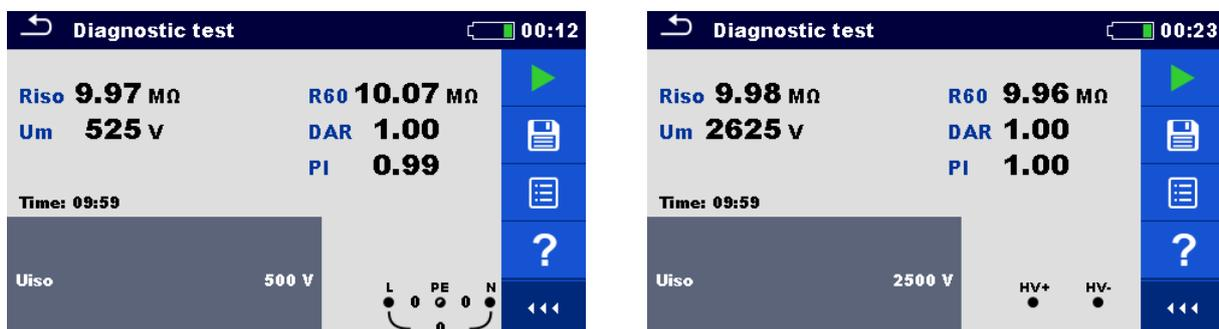
Figure 7.13: Examples of Diagnostic test result
