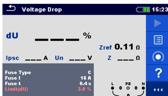
Figure 7.46: Example of Zref measurement result (STEP 1)
