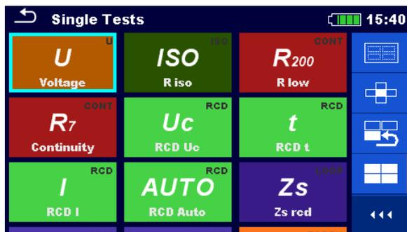
A single test can be selected from a list of all single tests.
