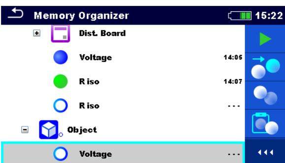
A new (empty) measurement is displayed in selected Structure object.
