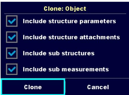
The Clone Structure object menu is displayed. Sub-elements of the selected structure object can be marked or un-marked for cloning.
