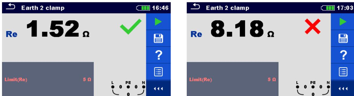
Figure 7.54: Examples of Contactless earthing resistance measurement result
