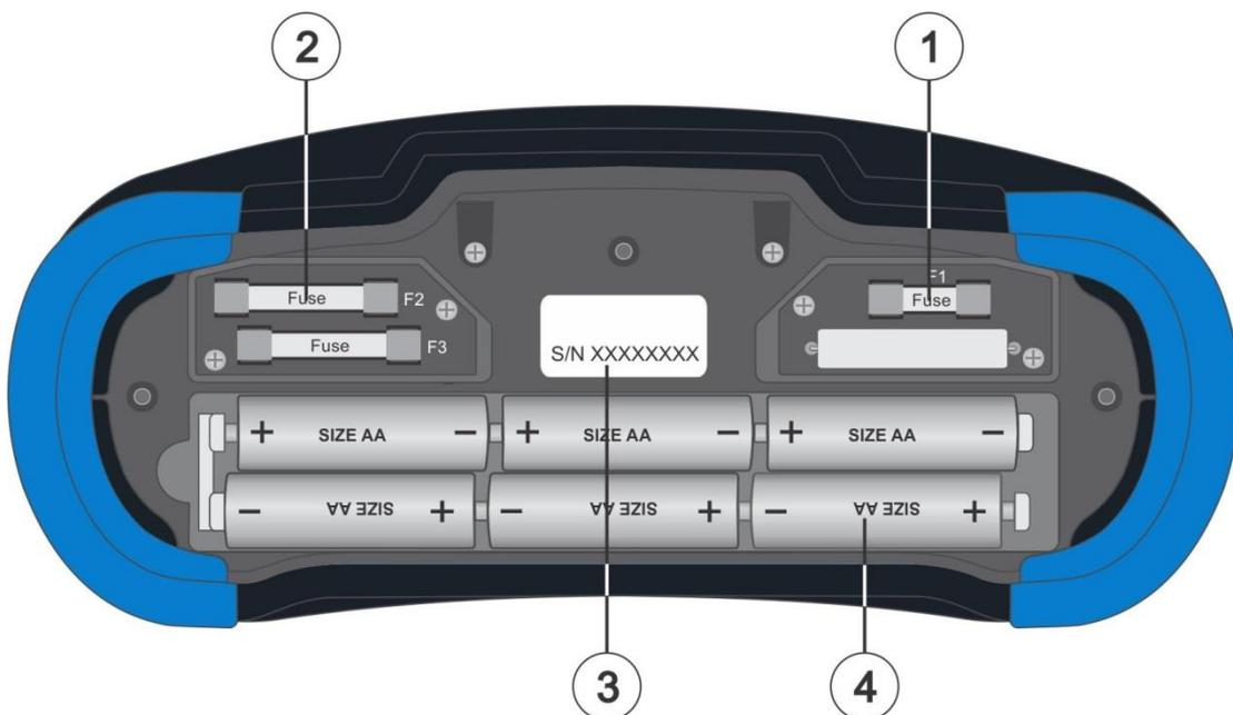
Figure 3.4: Battery and fuse compartment
