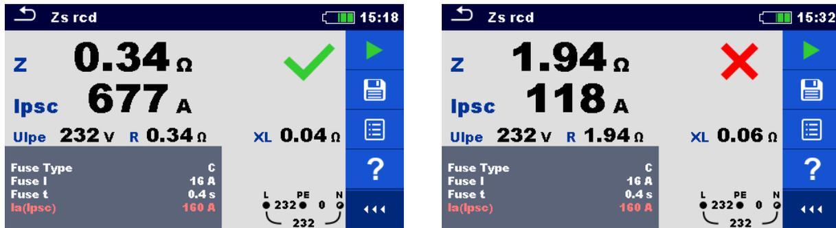
Figure 7.33: Examples of Zs rcd measurement result
