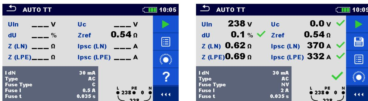
Figure 8.5: Examples of AUTO TT measurement results
