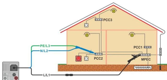
Figure 7.15: Connection of 3-wire test lead plus optional Extension lead
