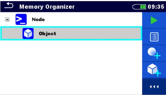
Select level in structure where measurement will be added.
