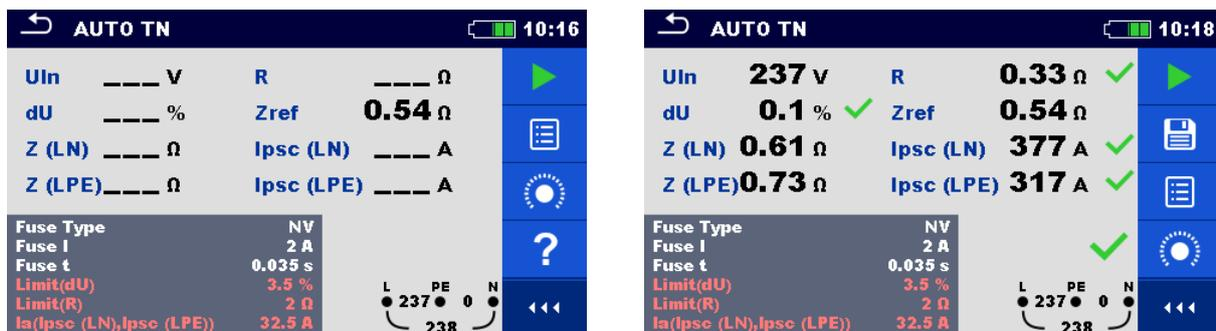
Figure 8.11: Examples of AUTO TN measurement results
