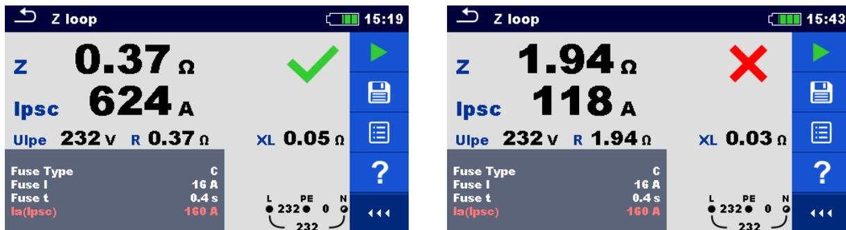
Figure 7.30: Examples of Loop impedance measurement result
