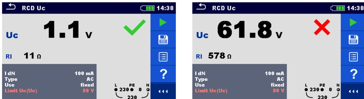
Figure 7.24: Examples of Contact voltage measurement result
