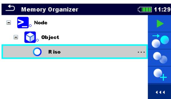
New empty measurement is added under the selected Structure object.
