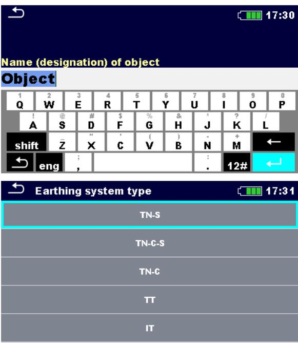
In menu for editing parameters the parameter's value can be selected from a dropdown list or entered via keypad. Refer to chapter **4 Instrument operation** for more information about keypad operation.
