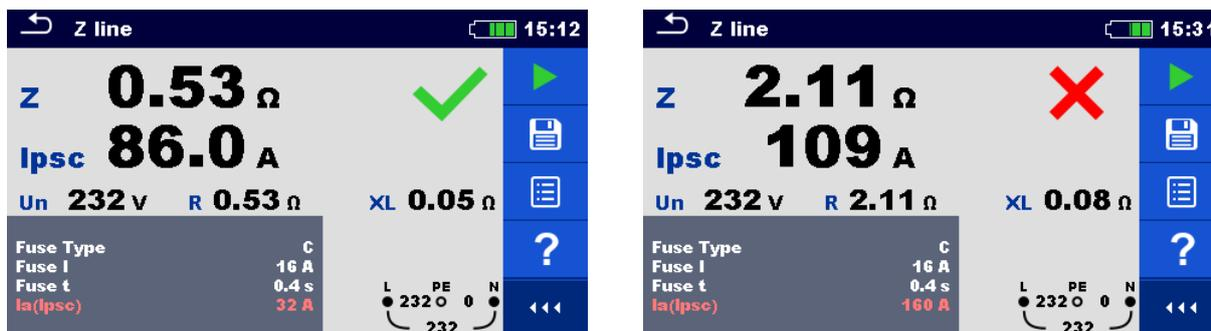
Figure 7.40: Examples of Line impedance measurement result
