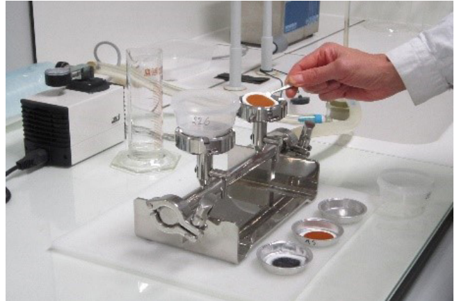
Detailed analysis of deposits or solids in the system water.
