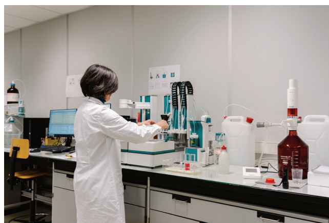
Titrator for the exact measurement of pH, conductivity and alkalinity.
