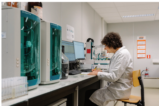
Ion chromatograph IC for the determination of various cations and anions.
