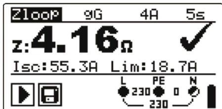
Figure 3.5: Typical function display
