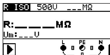
Figure 5.5: Insulation resistance
