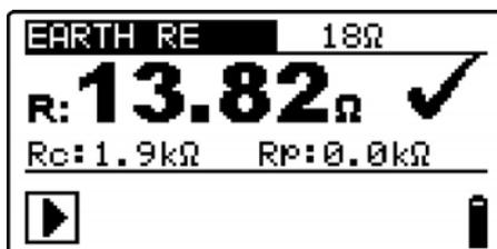
Figure 5.35: Example of earth resistance measurement result
