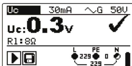
Figure 5.18: Example of contact voltage measurement results
