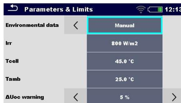
The manually entered environmental data will be used for calculation of STC results until they are updated (synchronized) with measured data from PV Remote WL.
