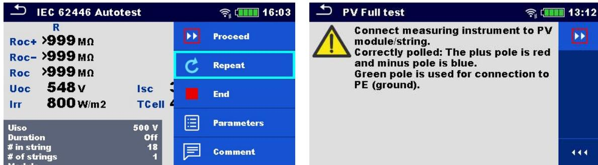
The offered options in the control panel depend on the selected single test, its result and the programmed test flow.
