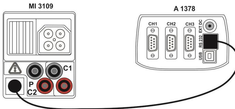
Figure 4.11: Connection of the instruments during synchronization
