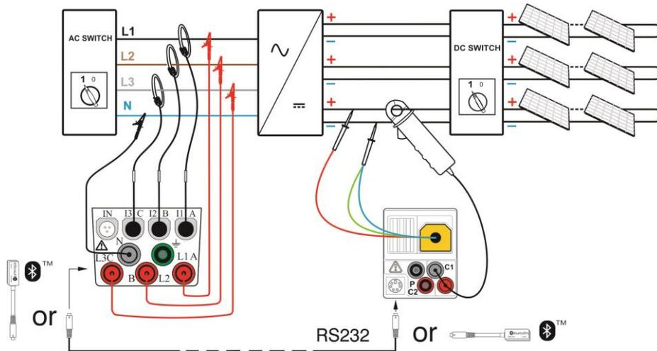
Figure 5.21: Connection in AC3 / DC sub-function using universal PV test lead
