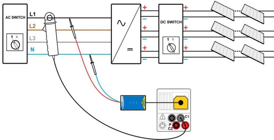
Figure 5.18: Connection with PV Safety Probe - AC side
