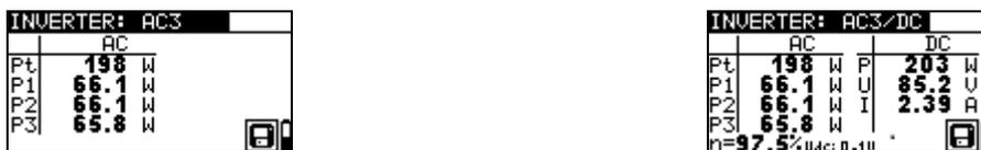
Figure 5.24: Examples of PV inverter test results screens - 3 phase a.c. output
