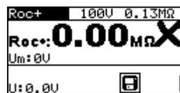
Figure 5.4: Examples of insulation resistance measurement result
