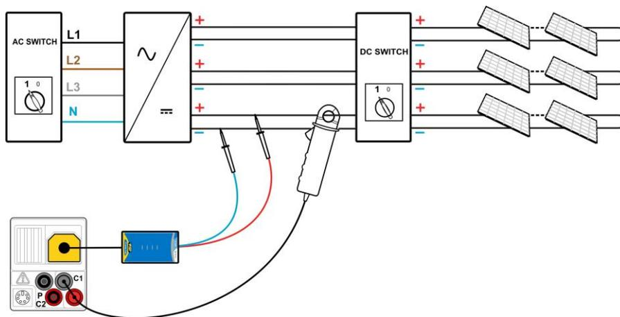
Figure 5.17: Connection with PV Safety Probe - DC side
