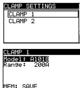
Figure 4.9: Configuration of current clamp measuring inputs
