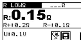
Figure 5.7: Example of RLOW  $\Omega$  result
