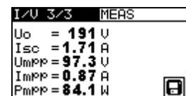
Figure 5.41: Example of I / V curve results
