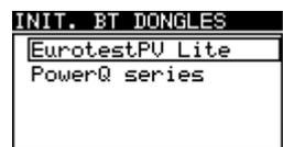
Figure 4.22: Menu for initialization of Bluetooth dongle(s)
