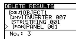
Figure 6.8: Clear measurements menu (data structure field selected)
