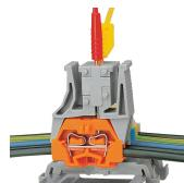
Testing via test plug modules snapped onto a terminal strip – wired or unwired. As touch contact is made with the CAGE CLAMP® (spring steel) unit, this testing type is limited to maximum 0.5 A.
