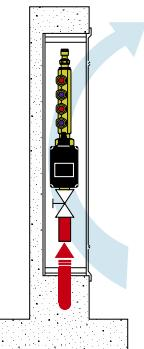
To prevent the formation of high temperatures where the zone valve is installed it is advisable to ensure a constant circulation of air.
