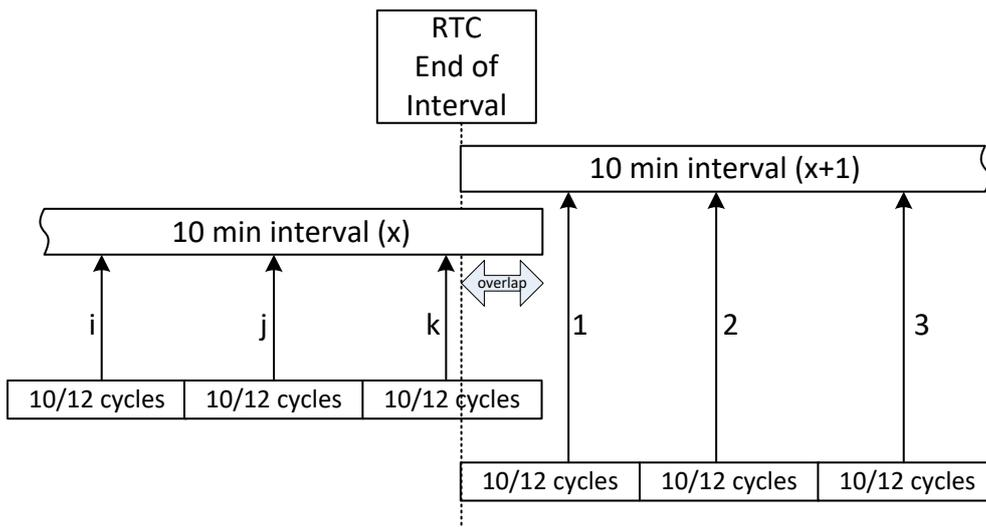
Figure 6.16: Synchronization and aggregation of 10/12 cycle intervals
