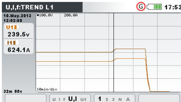
Figure 4.18: Voltage and current trend (single mode)
