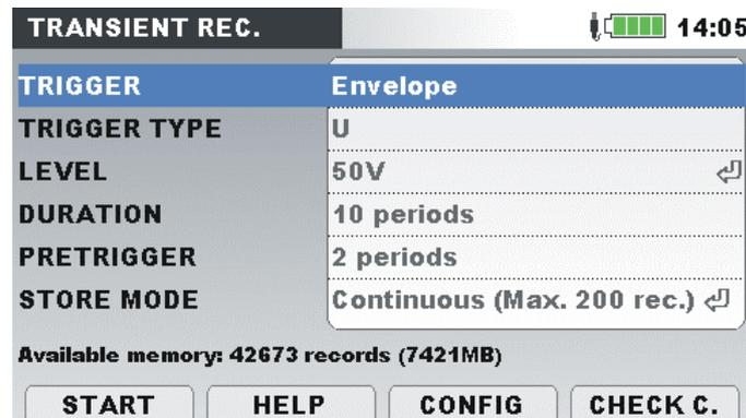
Figure 4.51: Transient recorder setup screen
