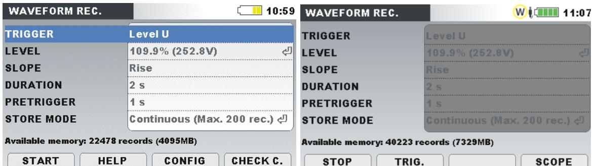
Figure 4.48: Waveform recorder setup screen
