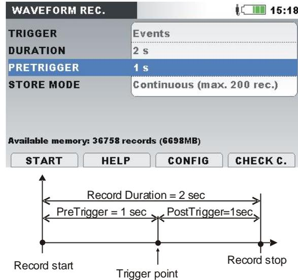
Figure 6.20: Triggering and pre-triggering description
