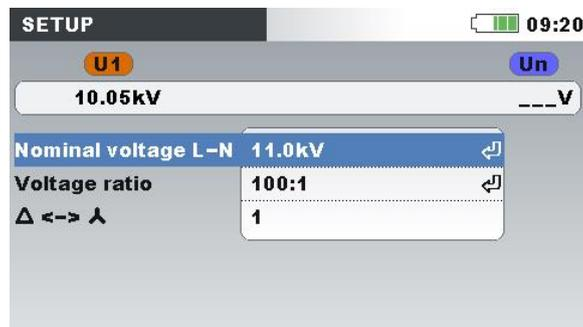
Figure 5.13: Voltage ratio for 11 kV / 110 kV transformer example
