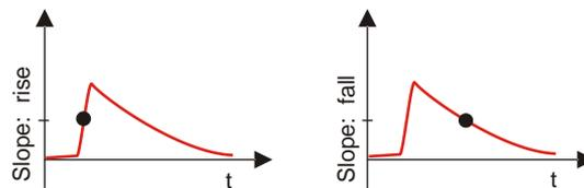
Figure 6.26: Triggering slope
