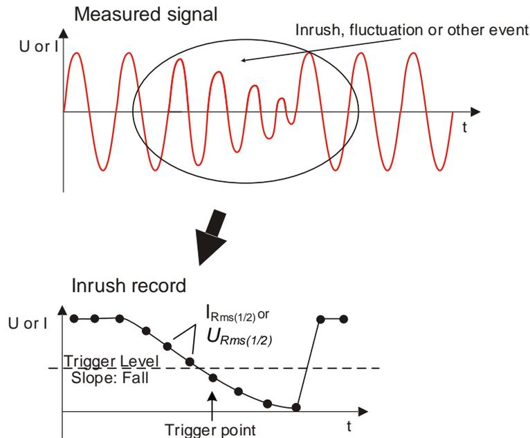
Figure 6.25: Level triggering
