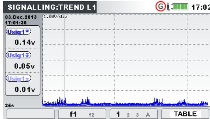
Figure 4.44: Signalling trend screen
