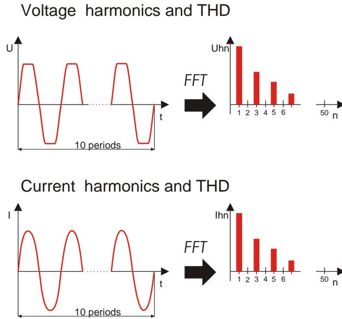
Figure 6.8: Current and voltage harmonics
