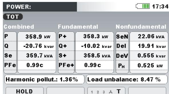
Figure 4.25: Detailed total power measurements
