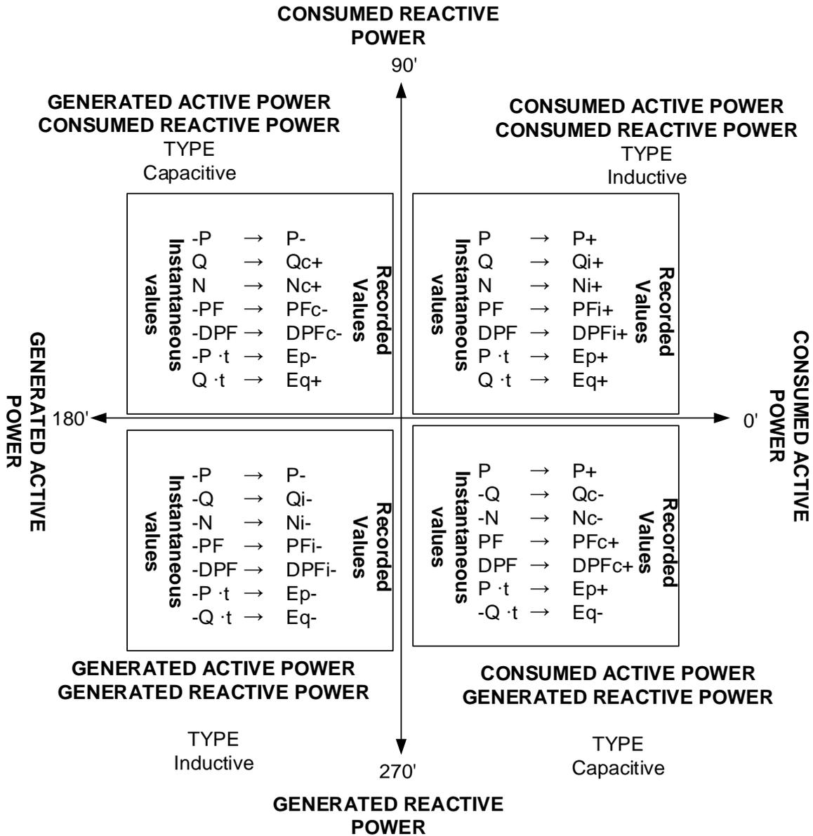
Figure 6.18: Consumed/generated and inductive/capacitive phase/polarity diagram
