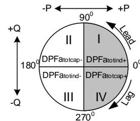
Instantaneous positive sequence total vector displacement (fundamental) power factor.
