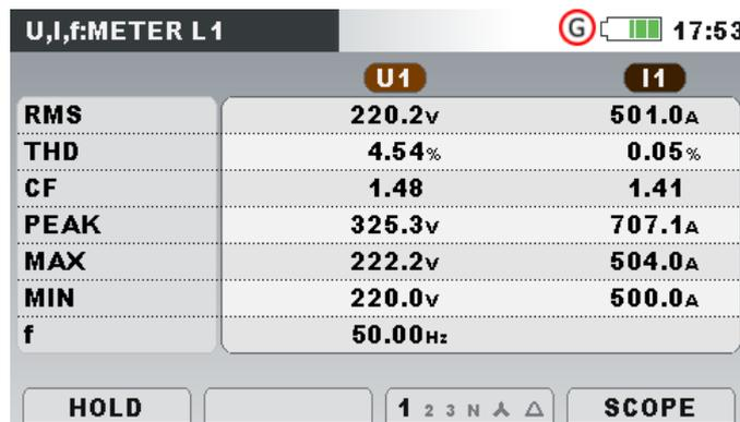
Figure 4.10: U, I, f meter phase table screens (L1, L2, L3, N)
