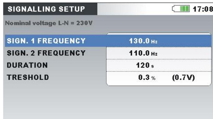
Figure 4.68: Signalling setup screen
