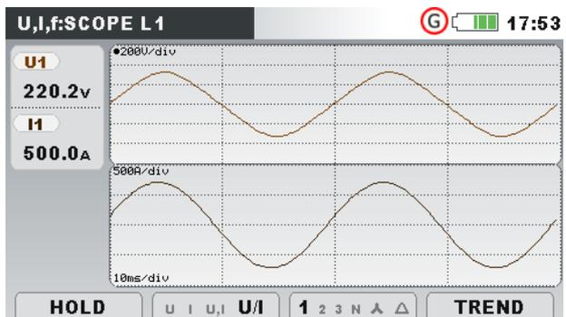
Figure 4.15: Voltage and current waveform (dual mode)
