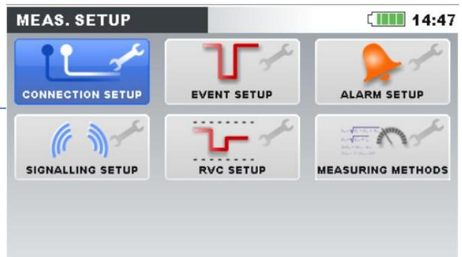
Figure 4.8: Measurement setup submenu
