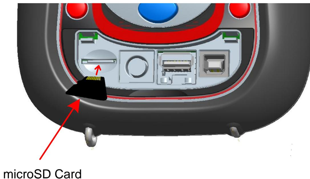
Figure 4.4: Inserting microSD card
