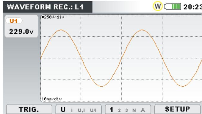
Figure 4.49: Waveform recorder capture screen
