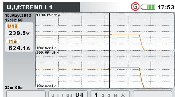
Figure 4.19: Voltage and current trend (dual mode)
