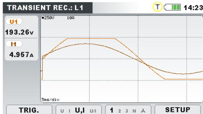
Figure 4.52: Transient recorder capture screen
