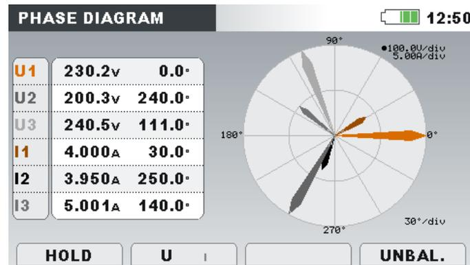
Figure 4.36: Phase diagram screen
