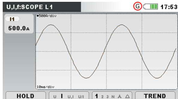
Figure 4.13: Current only waveform
