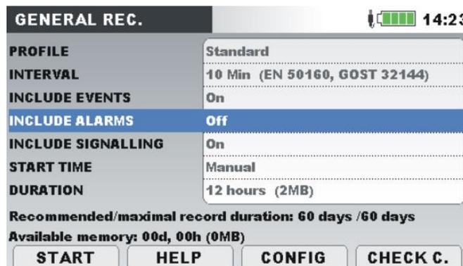
Figure 4.46: General recorder setup screen
