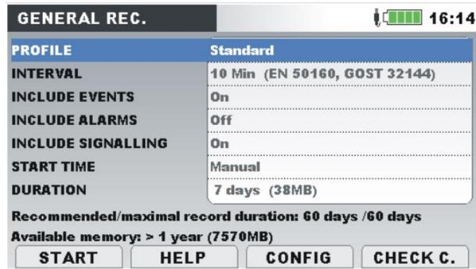
Figure 6.30: Predefined EN50160 recorder configuration
