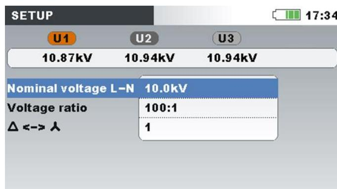
**Voltage ratio:** Potential transformer ratio  $\Delta \leftrightarrow \blacktriangle$ :
