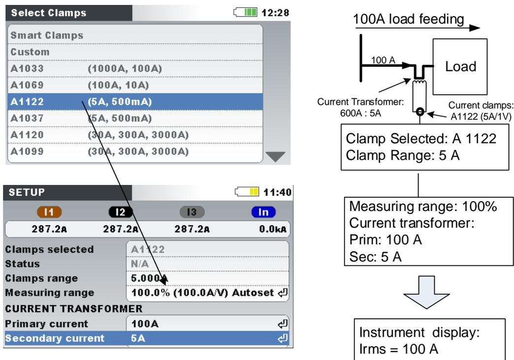
Figure 5.17: Current clamps selection for indirect current measurement
