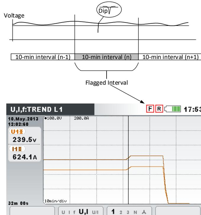
Figure 6.19: Flagging data indicate that aggregated value might be unreliable
