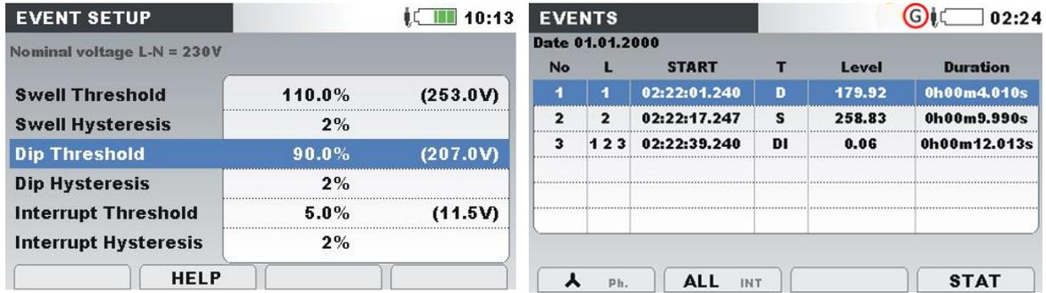
Figure 6.13: Voltage dip related screens on the instrument
