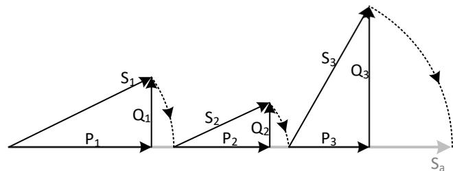
Figure 6.5: Arithmetic representation of total power calculus
