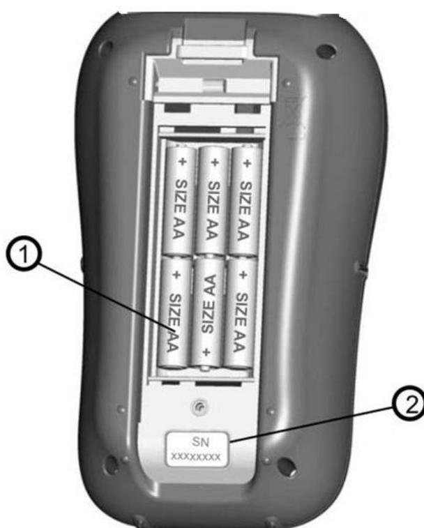
Figure 8.1: Battery compartment
