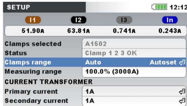
Figure 5.15: Smart current clamps auto range selection
