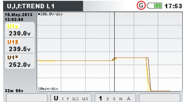
Figure 4.17: Voltage trend (single voltage)
