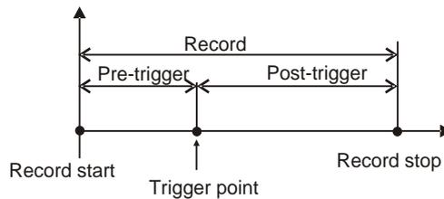
Figure 4.47: Triggering in waveform record
