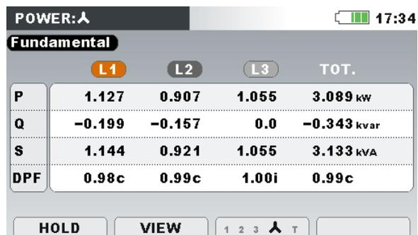
Figure 4.23: Power measurements summary (fundamental)
