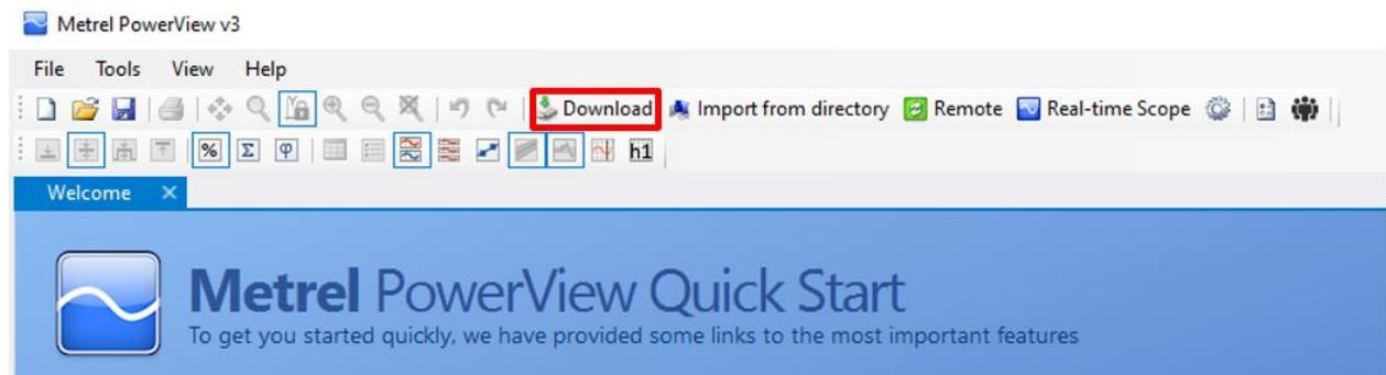
Download window will be displayed, and PowerView v3.0 will immediately try to connect to the instrument and detect the instrument model and firmware version.
