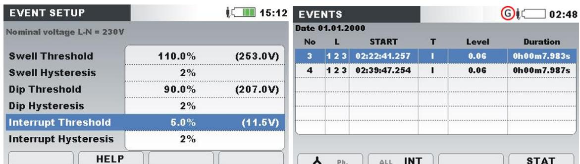
Figure 6.14: Voltage interrupts related screens on the instrument
