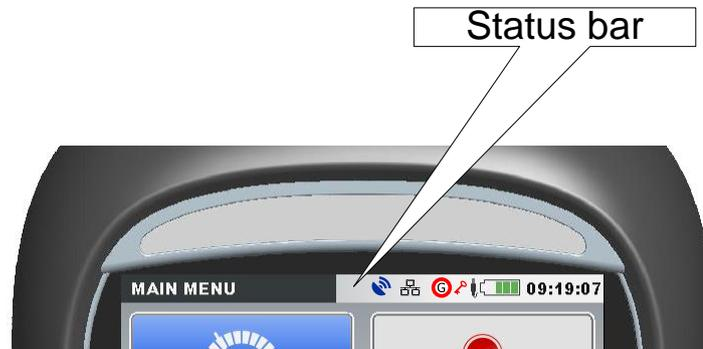
Figure 4.3: Instrument status bar
