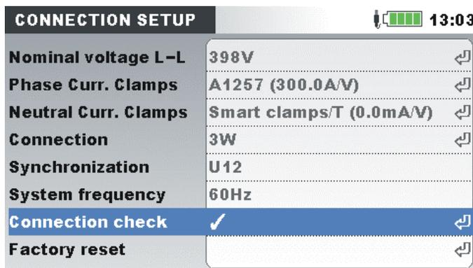
Connection check mark can be marked with OK (✓) or Fail (✗) sign and indicate overall connection status:
