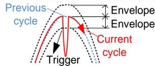
**Level:** Trigger will occur if any sample within period is greater than defined absolute trigger level. See 6.1.20 for details.
