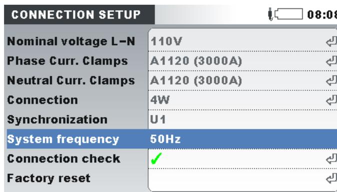
Figure 4.65: "CONNECTION SETUP" screen
