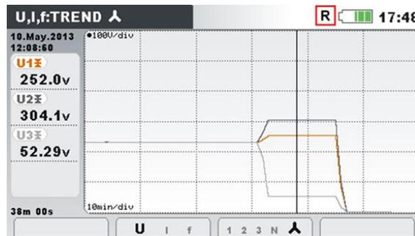
Figure 4.61: Viewing recorder U,I,f TREND data
