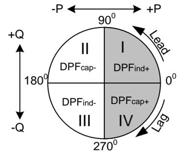
Instantaneous total arithmetic displacement (fundamental) power factor.
