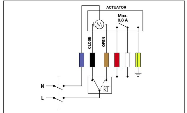
2. Connection diagram with ON/OFF switch interrupter.
