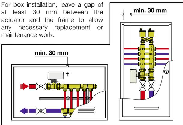
6. To prevent the temperature from becoming too high, make sure that air can circulate constantly around the zone valve.
