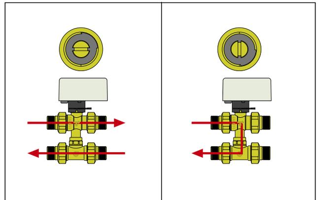
All the valves are supplied with the slot/indicator in the horizontal position.
