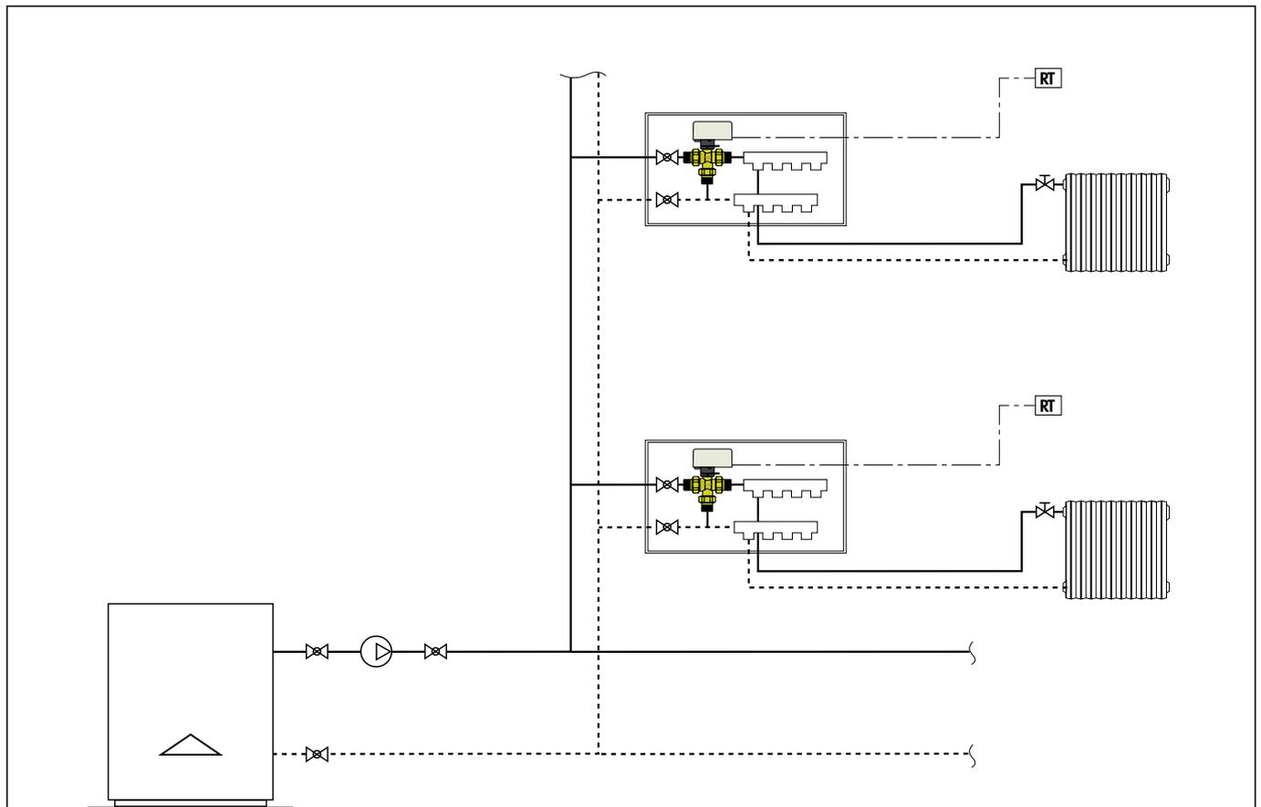
System with three-way zone valves with by-pass tee and AUTOFLOW®, 6444 series
