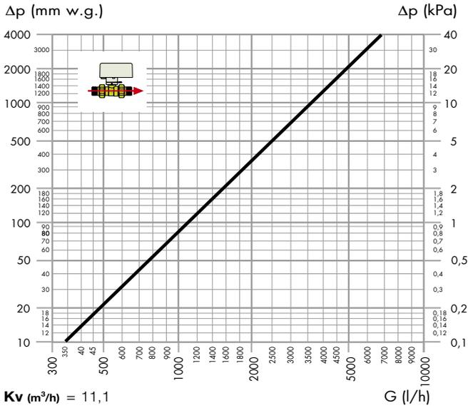
**6444 series three-way zone valve with by-pass in "open" mode, sizes 1/2", 3/4", 1"**
