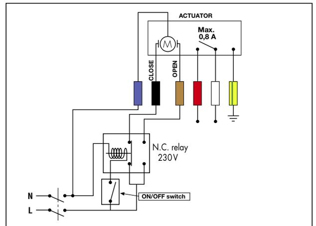
3. Diagram of pump deactivation when no zone is in operation.
