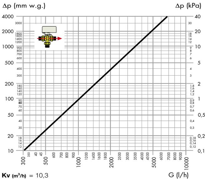
**6444 series three-way zone valve, in "by-pass" mode with U6 nozzle, sizes 1/2", 3/4", 1"**
