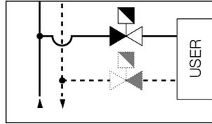
2. The three-way valves with by-pass and with by-pass tee must be installed on the flow pipe.
