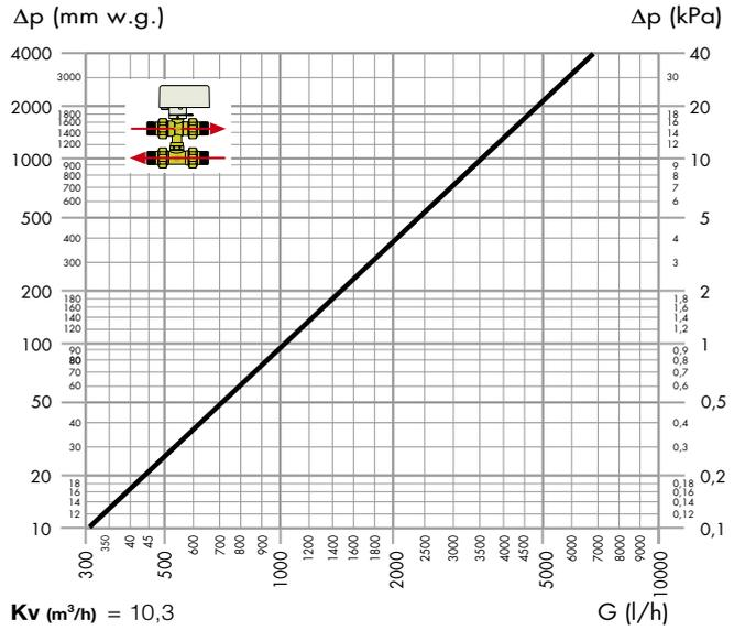
**Three-way zone valve with by-pass code 6443.. 3BY in "open" mode, sizes 1/2", 3/4", 1"**
