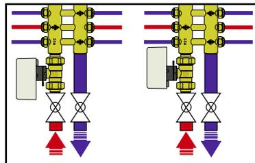
5. For box installation, leave a gap of at least 30 mm between the actuator and the frame to allow any necessary replacement or maintenance work.
