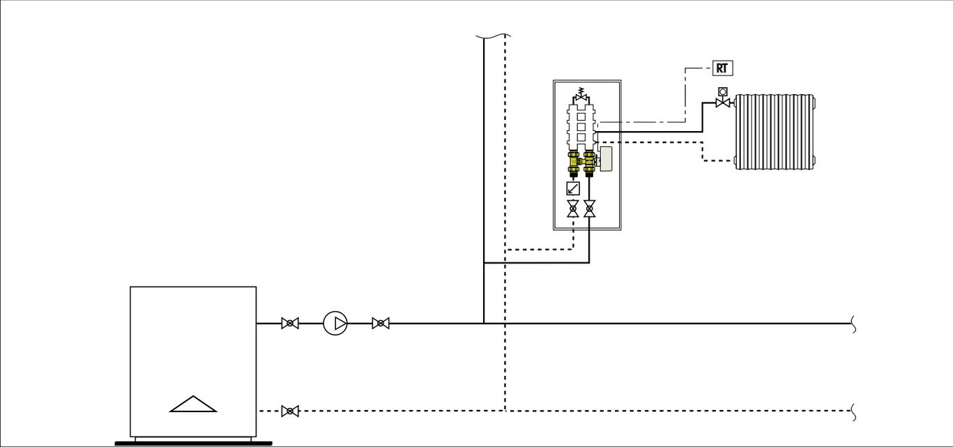
Independent system with three-way zone valves with by-pass tee and AUTOFLOW®, 6444 series
