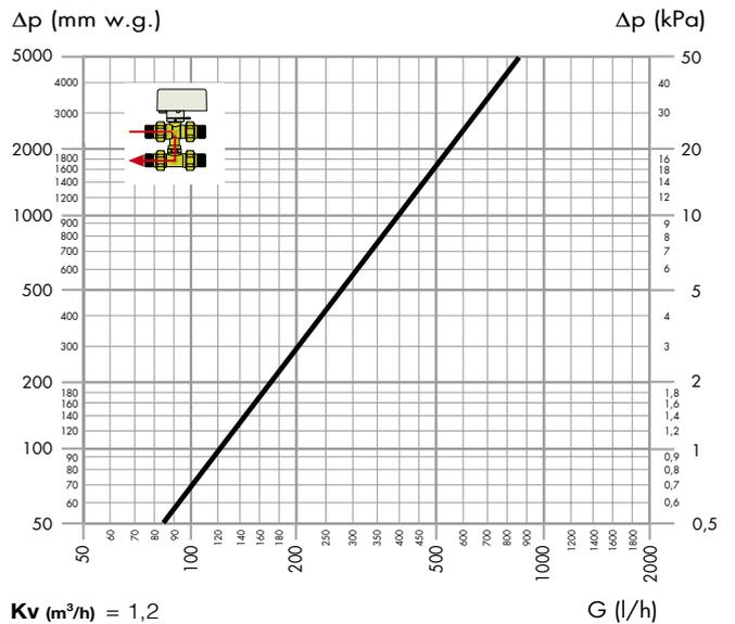
**Three-way zone valve with by-pass code 6443.. 3BY in "by-pass" mode, sizes 1/2", 3/4", 1"**
