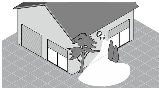
Fig. 25: Wall mounting on detached single-family house with floor lens 6851/22-xxx
