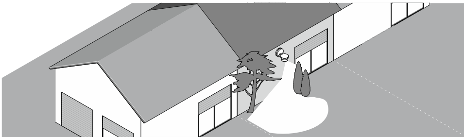
Fig. 23: Wall mounting on centre-row house for limited detection radius 6851/9-xxx
