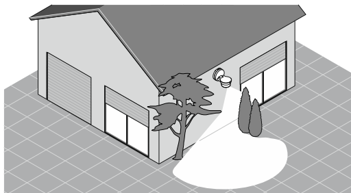
Fig. 25: Wall mounting on free-standing one-family house with bottom lens 6851/22-xxx
