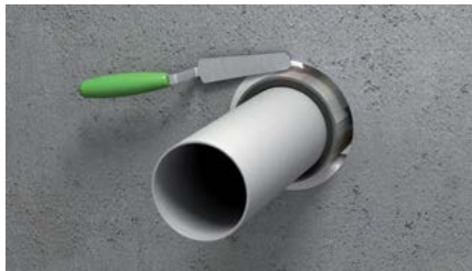
5. Ensure smoke tight seal of the annular gap. Seal it with a gap filler like Walraven Pacifyre® A acrylic sealant, Pacifyre® H hybrid sealant (fill depth = 10 mm) or Walraven Pacifyre® FPM fire protection mortar.
