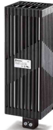
Type 7H.51.0.230.0150 Heater power 150 W Dimensions (w x h x d): 70 x 218 x 63 mm
