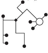
There are no restrictions for the network topology (star, ring, tree or mixed forms are permitted). Supply and communication in one and the same 3-wire cable • no shielding or twisting necessary • no terminating resistors required
