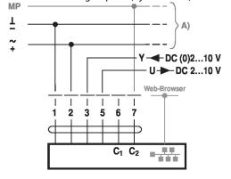
MP-Bus, supply via 3-wire connection
