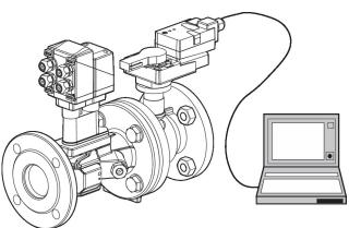
This can be inverted in cases of control with an analogue control signal DDC. The inversion causes the reversal of the standard behaviour, i.e. at a control signal DDC of 0%, regulation is to V'max or Q'max, and the valve is closed at a control signal DDC of 100%.
