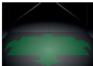
Room illumination with symmetric optics
