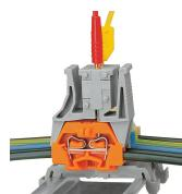
Testing via test plug modules snapped onto a terminal strip – wired or unwired. As touch contact is made with the CAGE CLAMP® (spring steel) unit, this testing type is limited to maximum 0.5 A.
