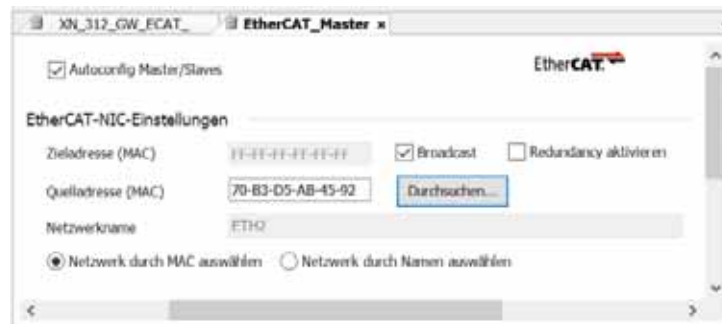
Figure 33: Configuring the Ethernet connection under the "General" tab for the EtherCAT master
