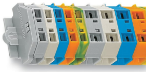
Terminal strip with mounting flanges, for screw or similar mounting types, 3.2 mm mounting hole diameter (with 209-123 Mounting Foot also for DIN-35 rail)
