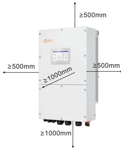
Figure 3.5 Inverter Mounting Clearances
