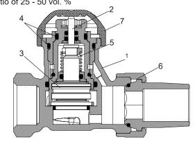
When using HERZ compression unions for copper and steel pipes, observe the permissible temperatures and pressures as specified in EN 1254-2:1998 Table 5. A maximum operating temperature of 95 °C and maximum operating pressure of 10 bar applies for plastic pipe connections, if permitted by the pipe manufacturer.
