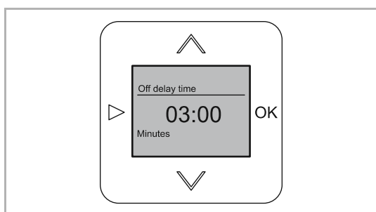
Fig. 12: Setup menu "Switch-off delay"
