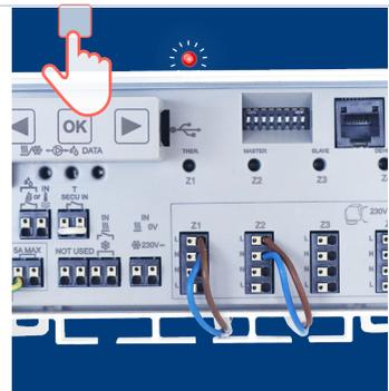
**Step 2** Confirm zone 1 by pressing **OK** - button to confirm that you want to pair a thermostat to pair.
