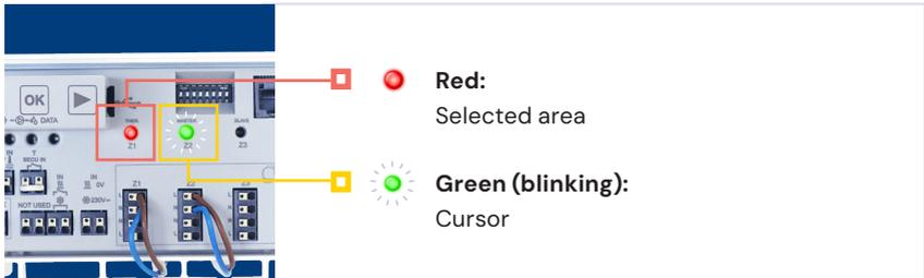
**Step 4** Now you can assign a thermostat to the selected zone. On the back of the thermostat there is a small button on the top left which you need to press with a small object.
