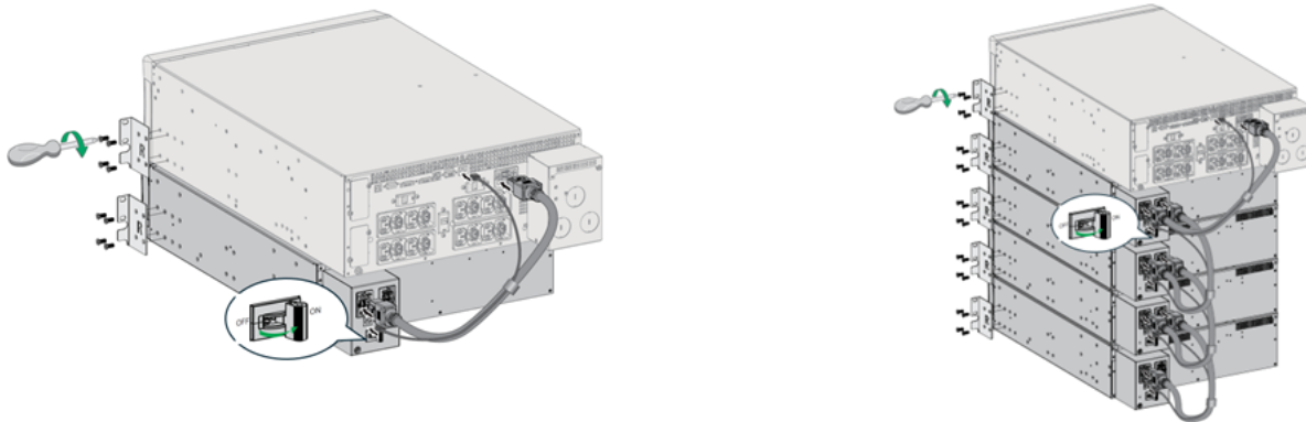
240V EBM connection to 8000VA and 11000VA UPS
