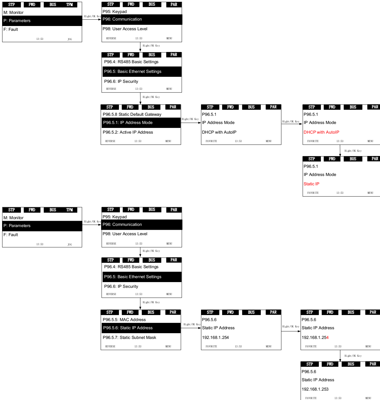
Figure 11. PowerXL DX1 Static IP mode
