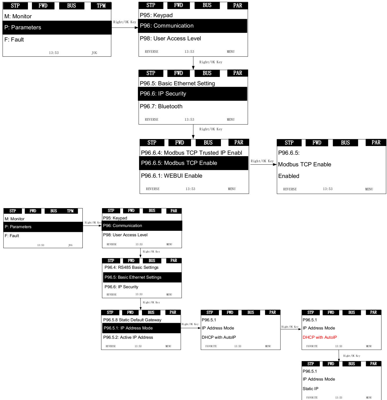
Figure 10. PowerXL DX1 keypad navigation to enable Modbus TCP
