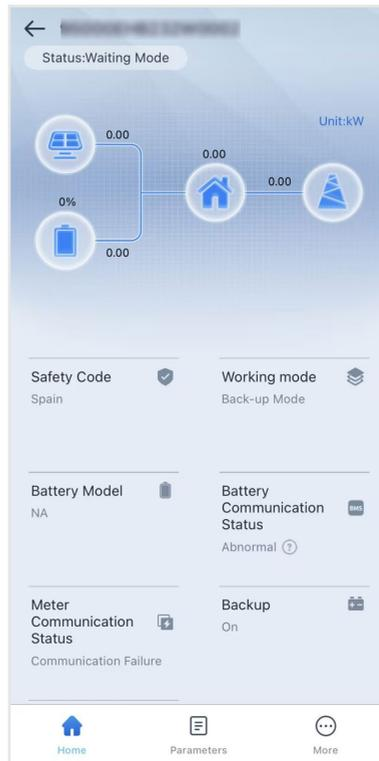
**Step 3:** Go to homepage, then click More>Quick Setting>BAT Access Mode>Battery Access to enter the parameter setting page. Follow the prompts on the interface to enter the battery model selection interface and set the battery model.
