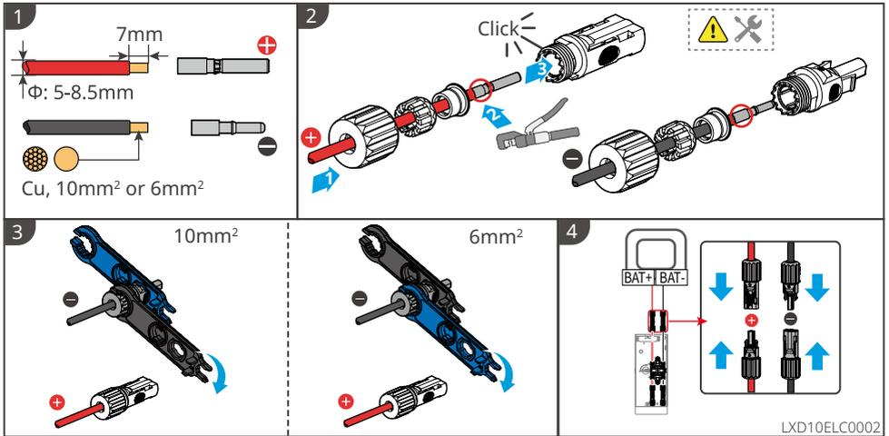
If you need to remove the power connector, please refer to the following steps and use the tools delivered with the box.
