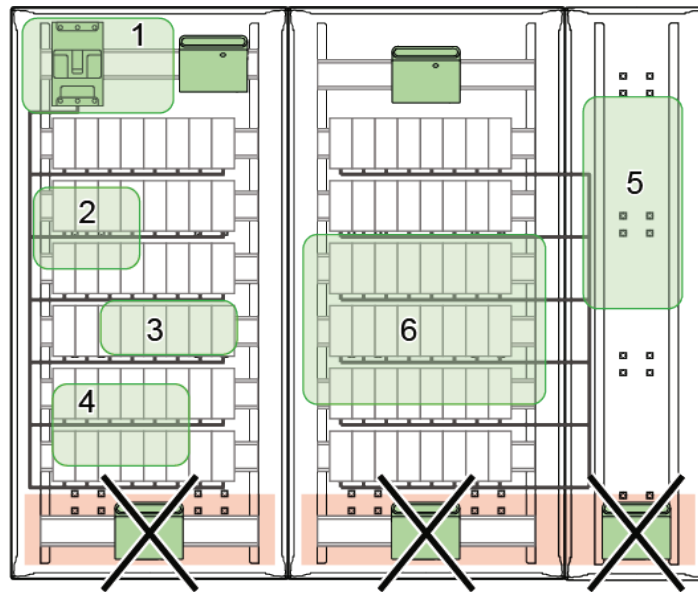
Illustration 17: Top Connection with several feeders in the incomer cubicle, and a dedicated FU cubicle with a cable cubicle
