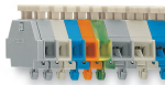
Terminal strip with snap-in mounting feet, for 0.6 ... 1.2 mm plate thickness, 3.5 mm mounting hole diameter (also for 210-154 Aluminum Rail or with 209-120 Mounting Foot for DIN-35 rail)
