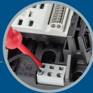
Tension clamp connection reduces the commissioning time
